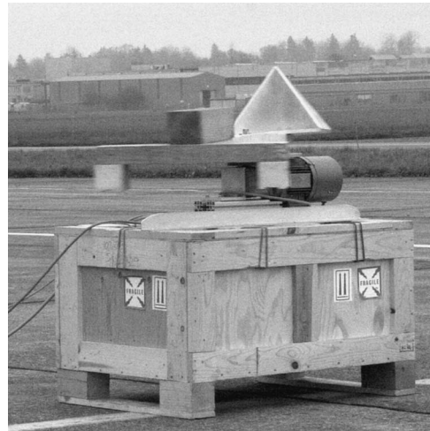
Fig. 16. Rotating corner reflector turning on a pedestal with 1 Hz.
